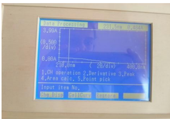
Fig. 3.2: Scan graph of cefpodoxime proxetil in phosphate buffer 6.8.
