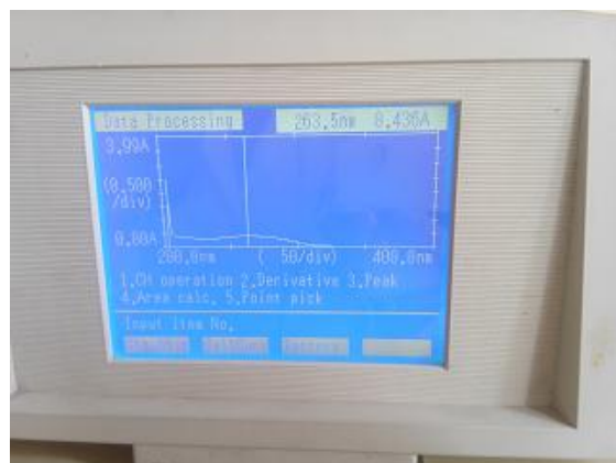
Fig. 3.3: Scan graph of cefpodoxime proxetil in pH 3.0 buffer.
