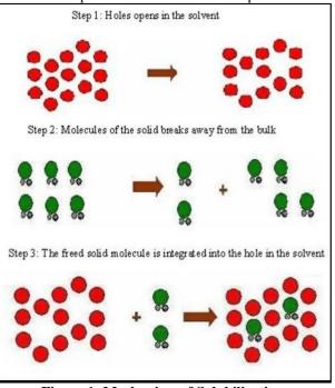
Figure 1: Mechanism of Solubilization.
