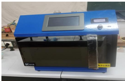
Fig. 1: Microwave Chemical Reactor FCMCR-3C-W (Gongyi City Kerui Instrument Co., Ltd).
