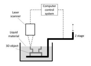
SLA functions through the precise exposure of a fine layer of photosensitive liquid resin to a UV laser in the x and y-axes, leading to the specific photopolymerization of these regions. After finishing one layer, the build platform gently descends by  $50-200 \ \mu\text{m}$ , accommodating the chosen resolution of the build, enabling the new liquid resin to smoothly cover the already solidified layer.
