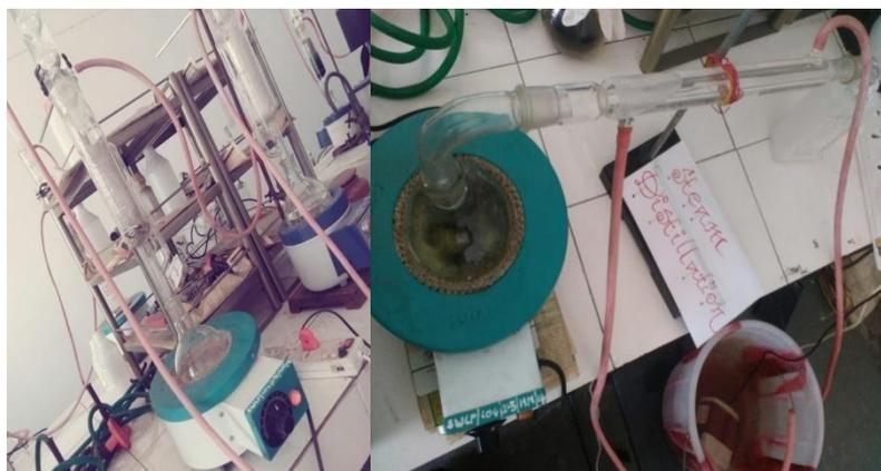
**Soxhlet Apparatus Steam distillation**
