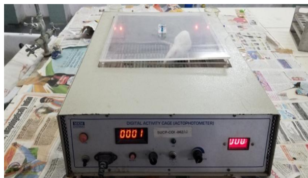
Figure 6: recording the locomotor activity using Actophotometer.
