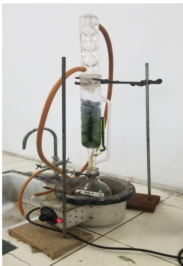
Figure 3: Preparation of extract using soxhlet apparatus.
