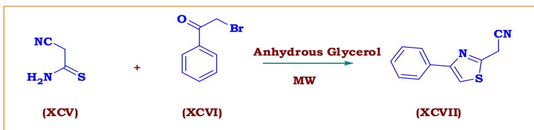
Scheme 1.2.6: Synthesis of thiazole derivative from thiocyno acetamide and 2-bromo-1-phenylethanone.
