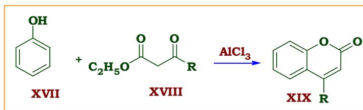
Scheme 1.1.2.1: Synthesis of 4-substituted coumarin by Pechmann condensation.
