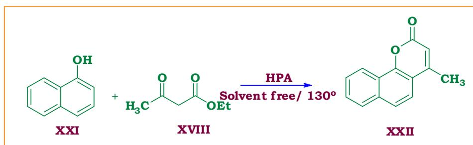
**Scheme 1.1.2.5: Synthesis of coumarin by pechmann condensation, in the presence of hetero poly acids.**
