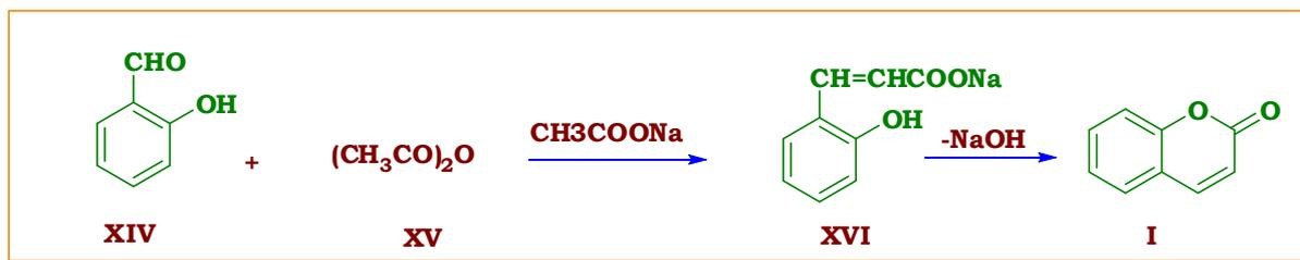
Scheme 1.1.1: Synthesis of simple coumarin by Perkin reaction.
