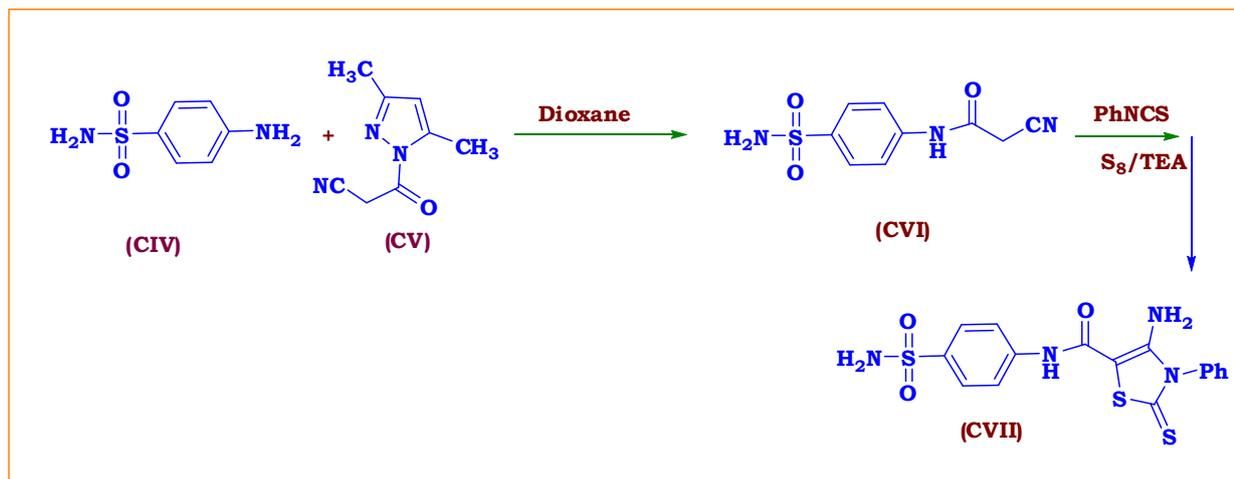
Scheme 1.2.9: Synthesis of thiazole derivative from pyrazole derivative with phenyl isothiocyanate.
