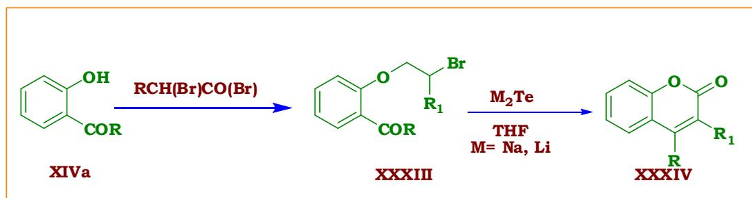
Scheme 1.1.5.2.: Synthesis of coumarin derivative in the presence of Na/Li-Te alloy.
