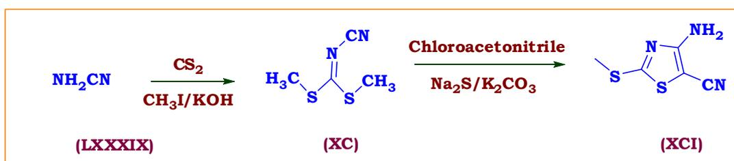
Scheme 1.2.4: Synthesis of thiazole derivative from compound (LXXXIX) reaction with carbon di sulfide.
