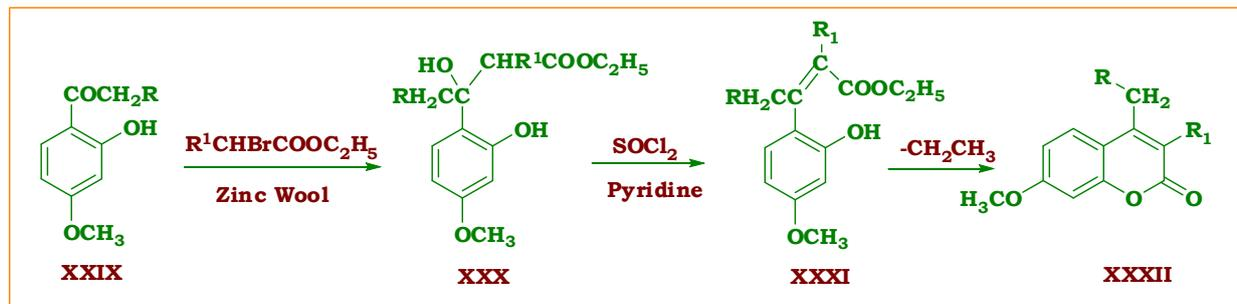
Scheme 1.1.5.1: Synthesis of coumarin derivative by Reformatsky reaction in the presence of thionyl chloride and pyridine catalyst.
