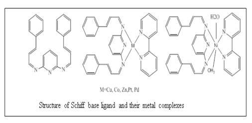
The metal complexes of Co (II), Ni (II), Cu (II) and Zn (II) with four heterocyclic Schiff base ligand synthesized.<sup>[23]</sup> such as,
