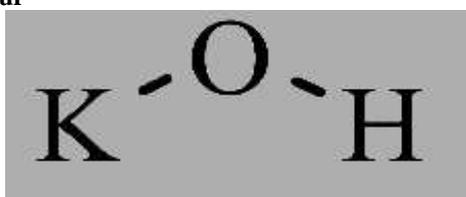
Potassium Hydroxide is an odorless, white or slightly yellow, flakey or lumpy solid which is often in a water solution. It is used in making soap, as an electrolyte in alkaline batteries and in electroplating, lithography, and
